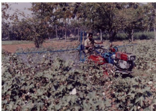
Fig. 3: Operational View in Power Tiller Operated Rear Mounted Boom Sprayer in Cotton Crop
