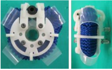
Fig. 2: Holding mechanism using extension type flexible pneumatic actuator
