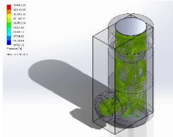
**Fig. 12:** Flow simulation.
