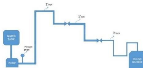
**Fig. 8:** Pipeline setup Fig.8 shows that general pipeline layout for the clean-in-process
