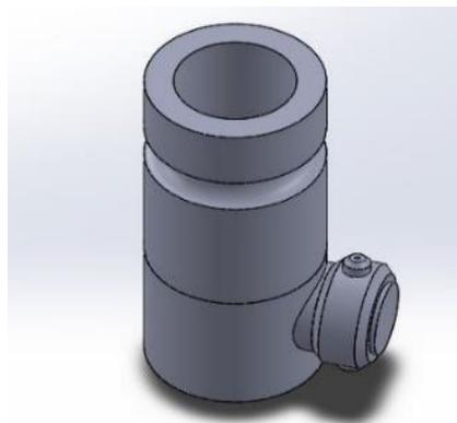
**Fig. 10:** Rotary Nozzle
