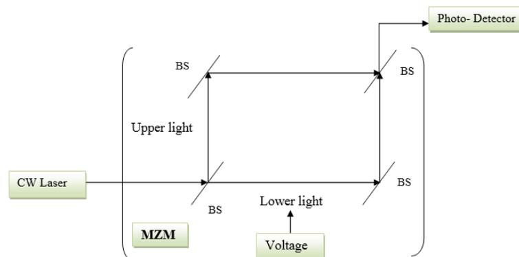
**Fig. 2:** Basic working model of a MZM
