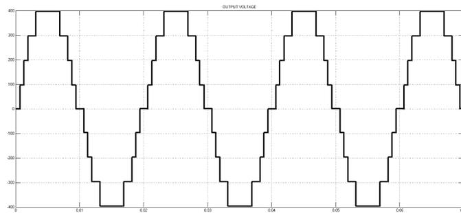
**Fig. 8:** Nine level output for proposed topology.
