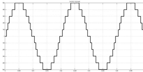
**Fig. 11:** Nine level output for proposed topology.
