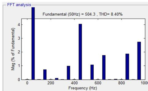
**Fig. 12:** Harmonics analysis of 9 level proposed topology.
