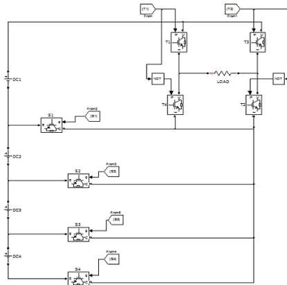
**Fig. 7:** Simulation diagram of 9 level proposed topology.
