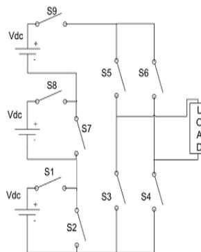
**Fig. 3:** Configuration of 7 level 9 switch topology.
