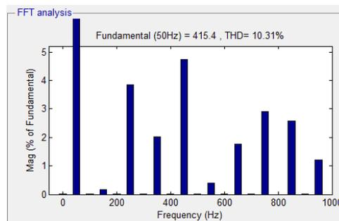
**Fig. 9:** Harmonics analysis of 9 level proposed topology.
