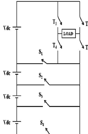
**Fig. 6:** Configuration of 9 level proposed Cascaded Multilevel Inverter.
