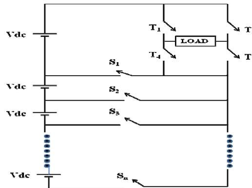
**Fig. 5:** Configuration of proposed Cascaded Multilevel Inverter.
