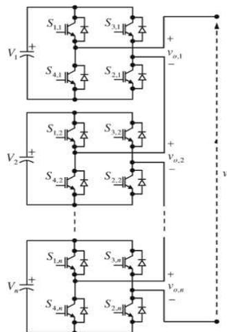
**Fig. 1:** Configuration of Cascaded H-Bridge Multilevel Inverter.
