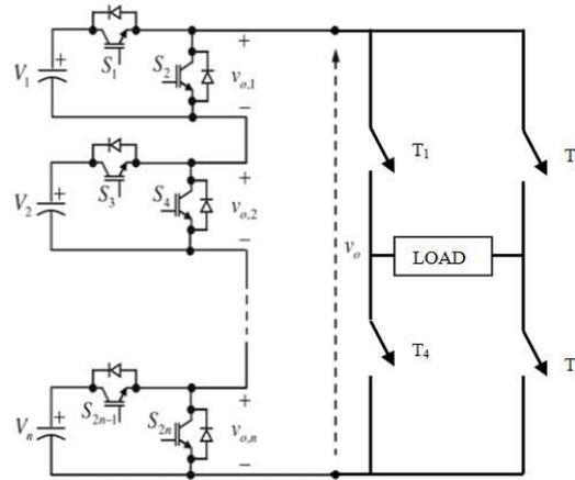
**Fig. 2:** Configuration of Existing Topology 1.
