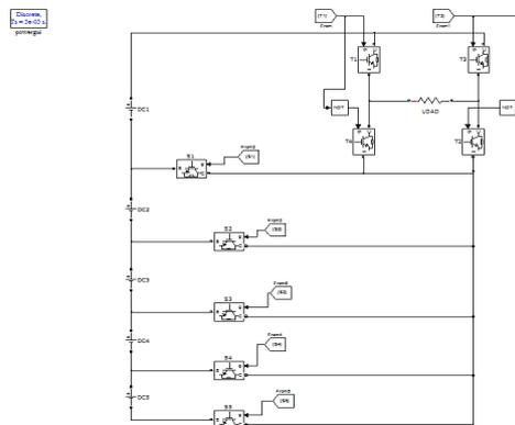
**Fig. 10:** Simulation diagram of 11 level proposed topology.
