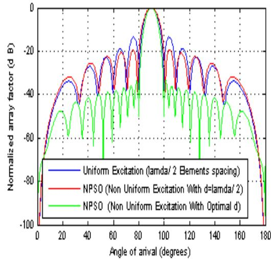
**Fig. 2:** Radiation pattern of 12 element half wavelength dipole antenna arrays with mutual coupling effect.
