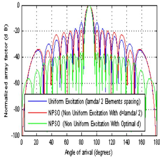
**Fig. 3:** Radiation Pattern of 16 element half wavelength dipole antenna arrays without including mutual coupling effect.
