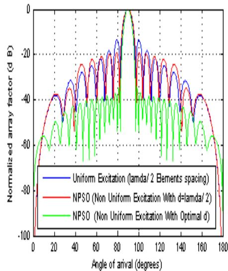
**Fig. 4:** Radiation Pattern of 16 element half wavelength dipole antenna arrays including mutual coupling effect.
