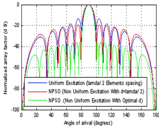
**Fig. 1:** Radiation Pattern of 12 element half wavelength dipole antenna arrays without mutual coupling effect.
