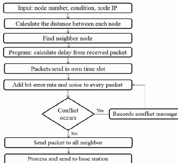
**Fig. 2:** Flow diagram of HRNC
