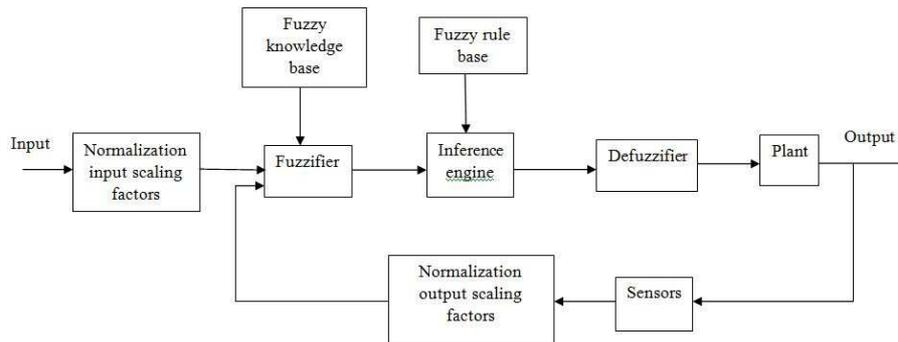
**Fig. 1:** General Block Diagram of Fuzzy Controller
