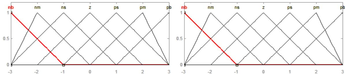
**Fig. 3:** Input membership function for e and ec
