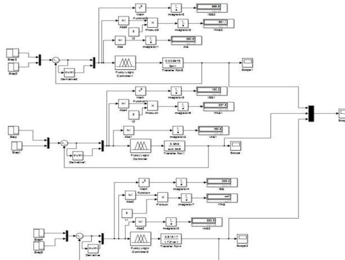
Fig. 5: Simulation block diagram for heat exchangers
