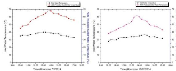
Fig. 4: Inlet and outlet water temperature variation with respect to time.
