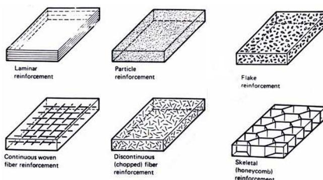
**Fig. 2:** illustration of composite reinforcement common thermosetting resin matrix materials are phenolic, epoxy and polyester resins.
