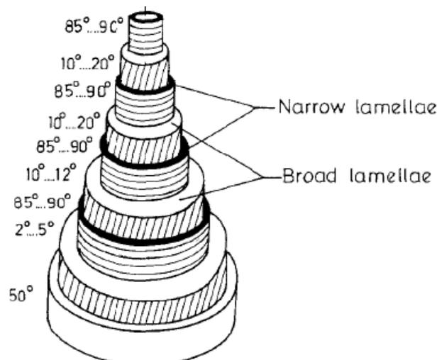
Fig. 1: Structure of Bamboo
