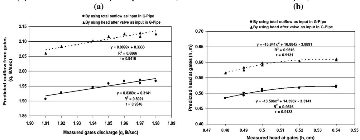
**Fig. 6:** (a) Relationship between measured and predicted outflow from gates ( $q$ , L/sec) (b) relationship between measured and predicted head ( $h$ , m), along gated pipeline (6 m length and 8 gate) under zero slope of pipeline by using two different G-pipe simulation model as a primary conditions (total outflow or head after valve inputs).
