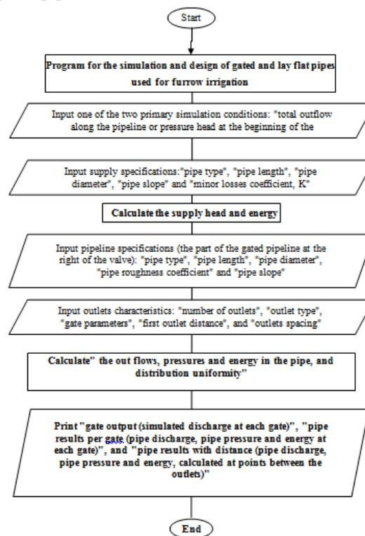
**Fig. 2:** Flow chart components of G-Pipe simulation model program for simulating outflow and pressure at gates along the pipeline of gated pipes irrigation system.
