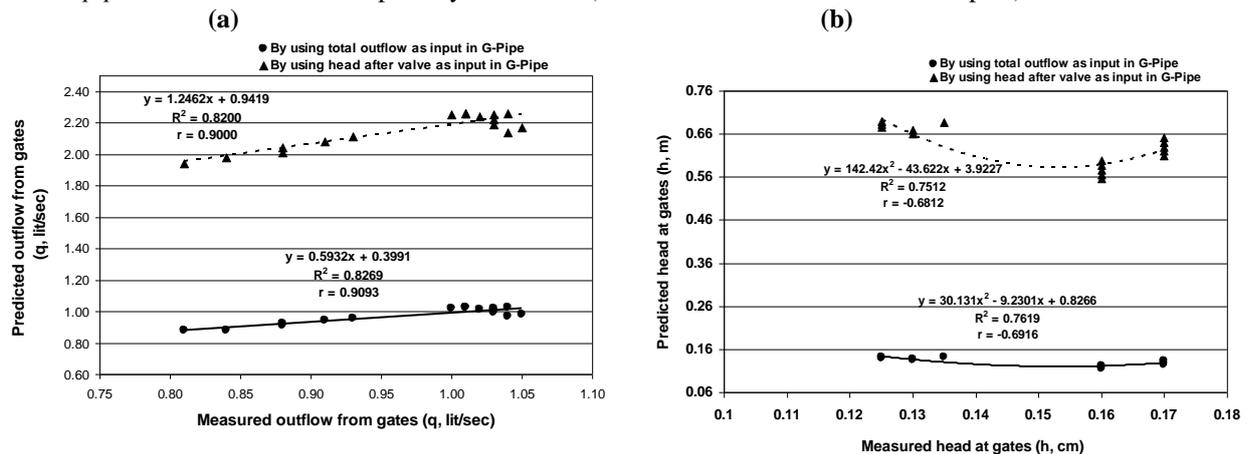
**Fig. 4:** (a) Relationship between measured and predicted outflow from gates (q, lit/sec) (b) relationship between measured and predicted head at gates (h, m), along gated pipeline (12 m length and 16 gates) under zero slope of pipeline by using two different G-pipe simulation model as a primary conditions (total outflow or head after valve inputs).
