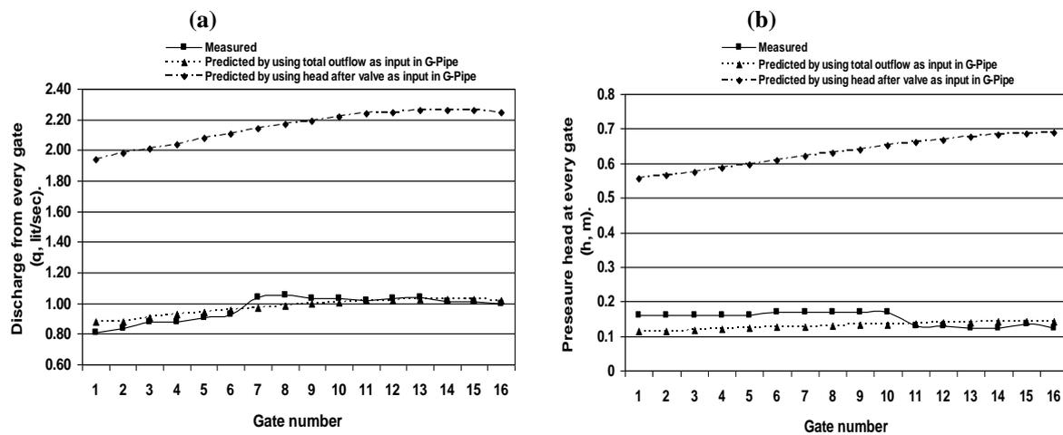
**Fig. 3:** (a) Measured and predicted discharge from every gate (b) Measured and predicted head at every gate, along gated pipeline (12 m length and 16 gates) under zero slope of pipeline by using two different G-pipe simulation model as a primary conditions (total outflow or head after valve inputs).
