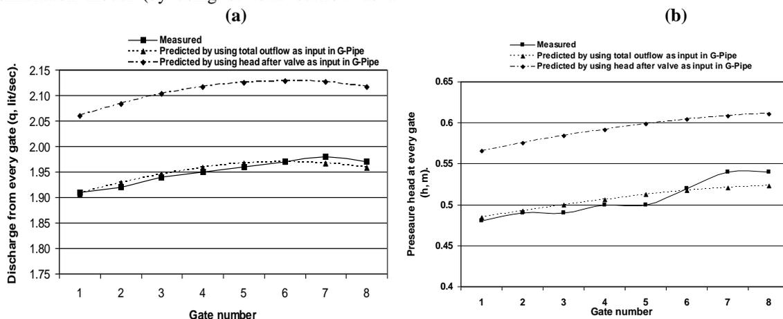
**Fig. 5:** (a) Measured and predicted discharge from every gate (b) Measured and predicted head at every gate, along gated pipeline (6 m length and 8 gate) under zero level of the pipeline by using two different G-pipe simulation model as a primary conditions (total outflow or head after valve inputs).
