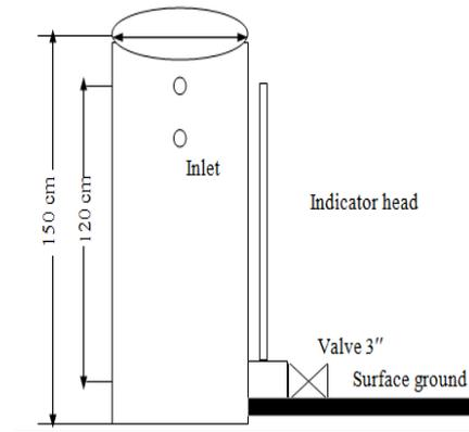
**Fig. 1:** Tank for calibration of gated pipe.
