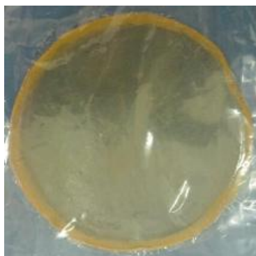
Fig. 1: Yellowish-translucent PBE film obtained via solution casting technique.
