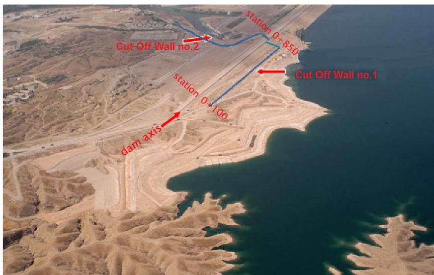
**Fig. 6:** Cut off walls No.1 and No.2 in left side.
