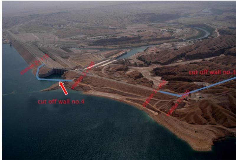
**Fig. 7:** Cut off walls No.3 and No.4 in right side.
