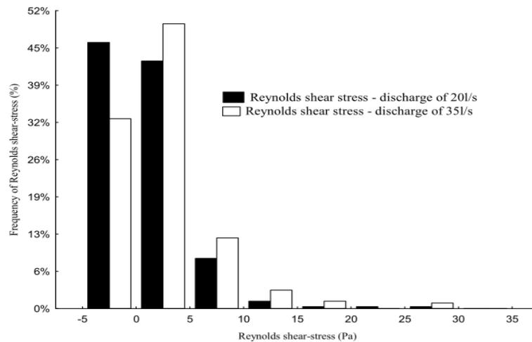
**Fig. 5:** Reynolds shear stress for discharge 20 L/S and 35 L/S.
