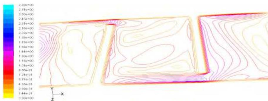
**Fig. 2:** Speed lines in the fourth fishway pool.
