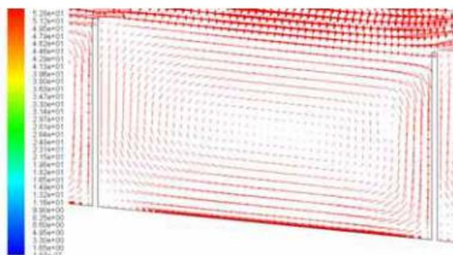
**Fig. 3:** Velocity vectors in the fishway pool.
