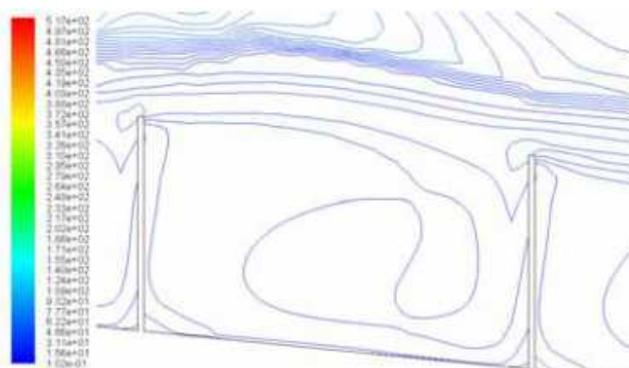
**Fig. 4:** Contours of turbulence intensity.
