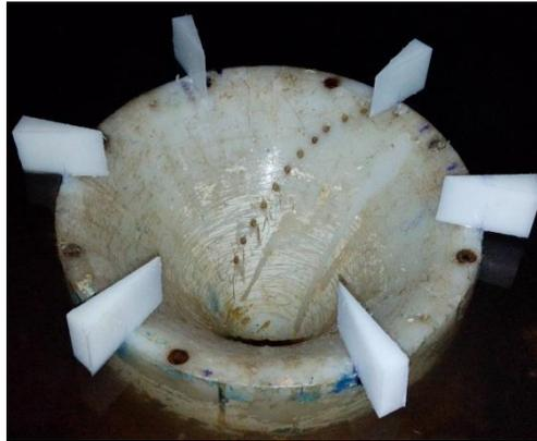
**Fig. 7:** A view of the position of triangular vortex breaker for length with a ratio of ( $L/D = 0.2$ )
