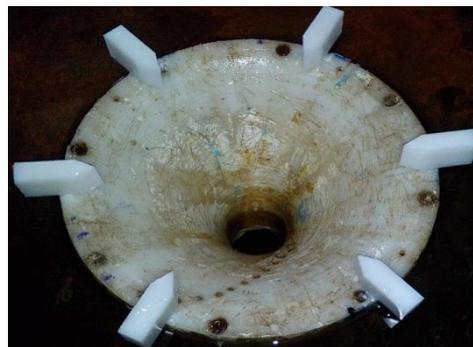
**Fig. 8:** A view of the position of sharp vortex breaker with the rectangular body for length ratio ( $L/D = 0.2$ )
