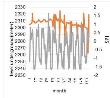
**Diagram 2:** estatical level average and severity of drought(2002-2012).
