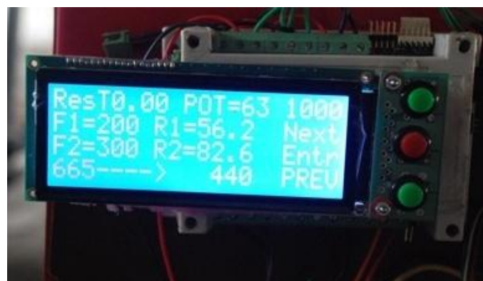
Fig. 7: The electronic control unit while measuring time lag
