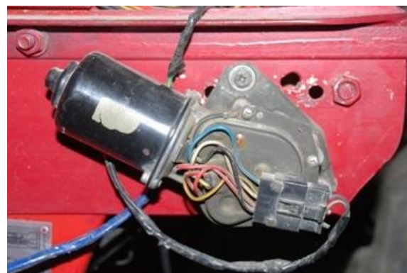
Fig. 3: Opening actuator (electromotor) of fertilizer meters.
