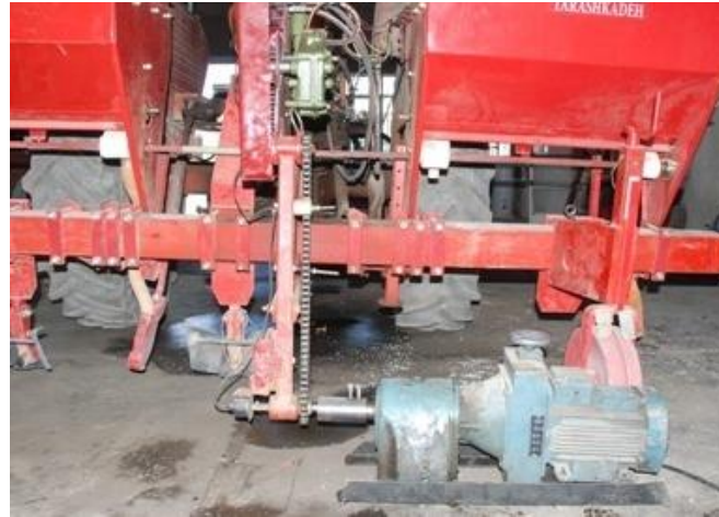
Fig. 6: The gearbox and electromotor collection replaced for the ground-driven wheel
