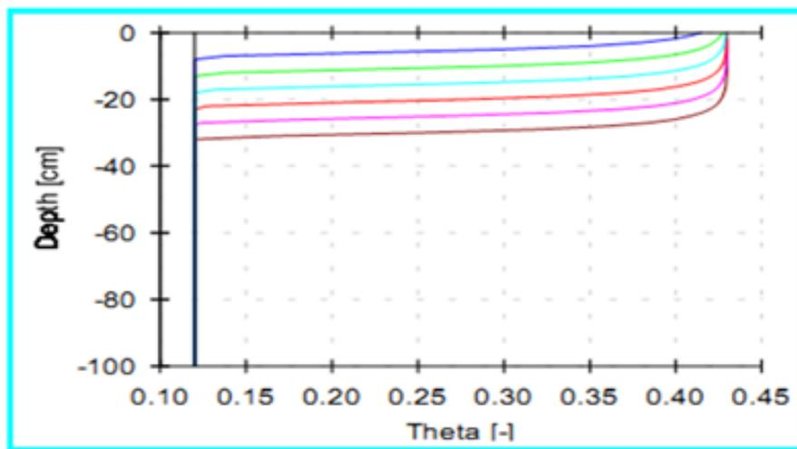
Fig. 6: Changes in soil moisture content at different times.
