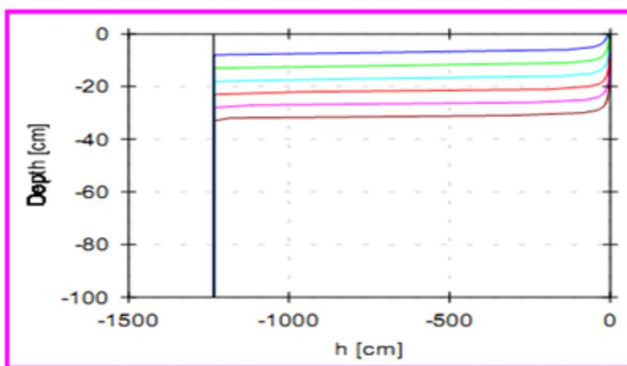
Fig. 7: Suction changes with soil depth at different times.
