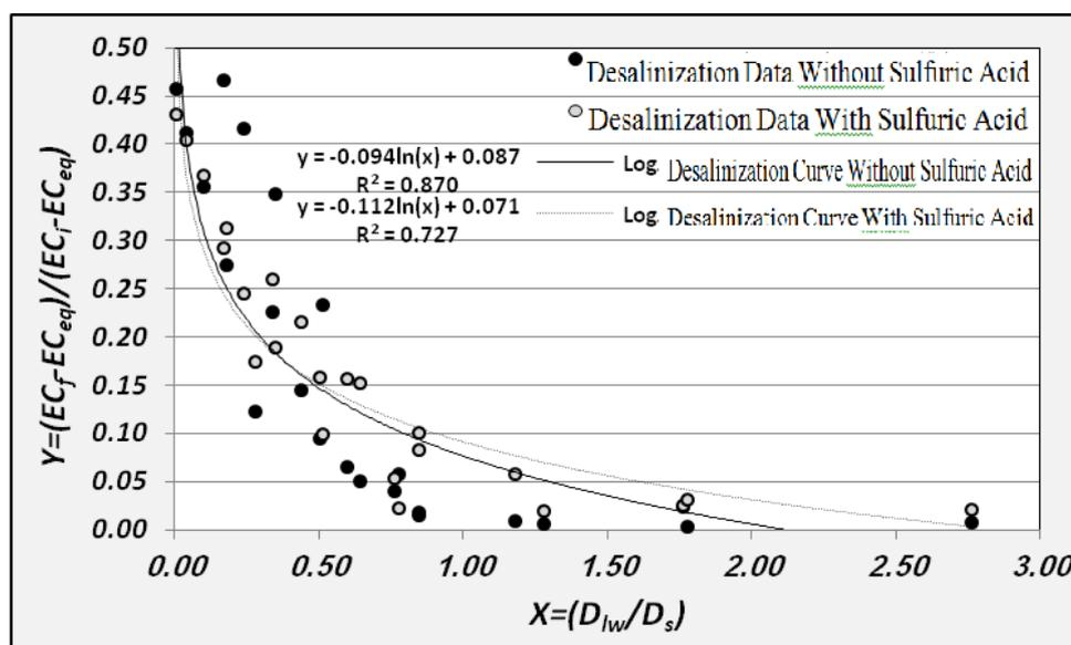
**Fig. 1:** Soil desalination curves under the influence of two leaching treatments in Deylam soil series.
