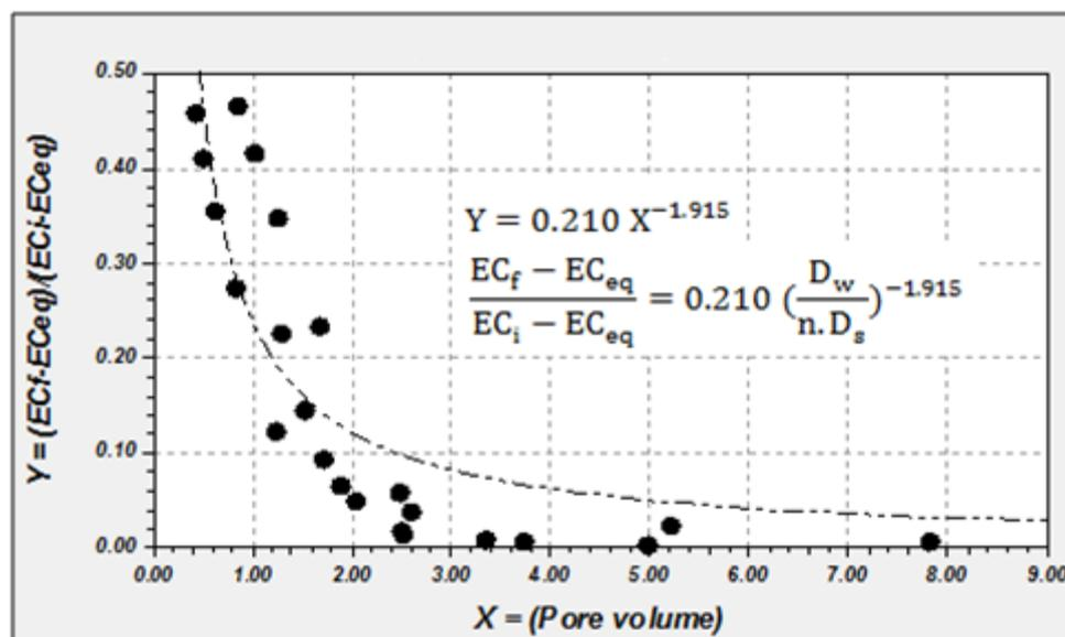
Fig. 2: Soil desalination curves versus different amounts of pore water in Deylam soil series (without reclamation substance).
