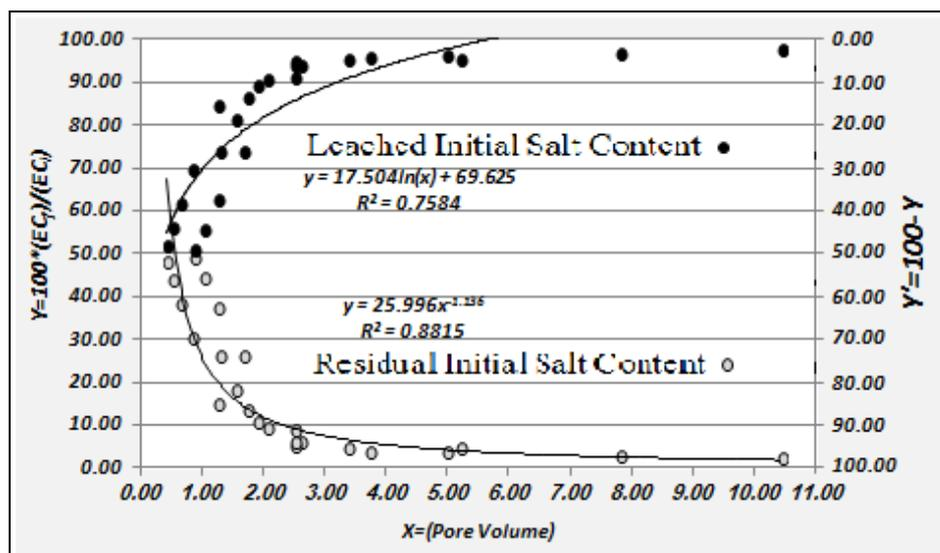
**Fig. 4:** Variation of initial removed and remained salts to pore porosity after leaching process in Deylam soil series (without reclamation substance).
