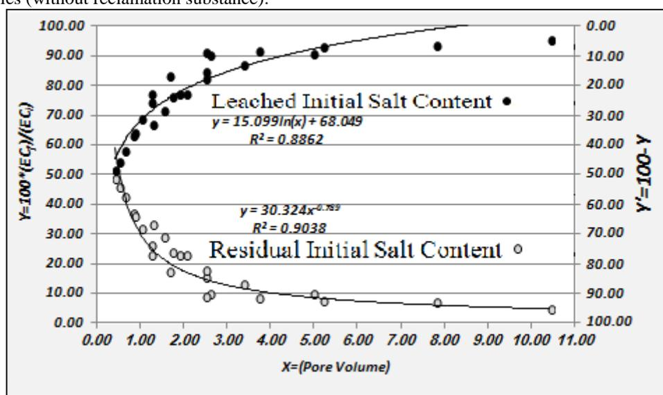
**Fig. 5:** Variation of initial removed and remained salts to pore porosity after leaching process in Deylam soil series (with reclamation substance).
