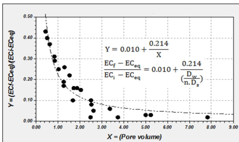
Fig. 3: Soil desalination curves versus different amounts of pore water in Deylam soil series (with reclamation substance).
