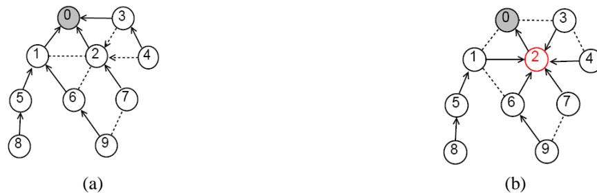
**Fig. 1:** a) Sensor network before being attacked by sink hole b) Sensor network after being attacked by sink hole [12].
