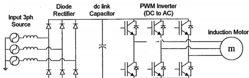
**Fig. 5:** Typical adjustable speed drive (ASD) system
