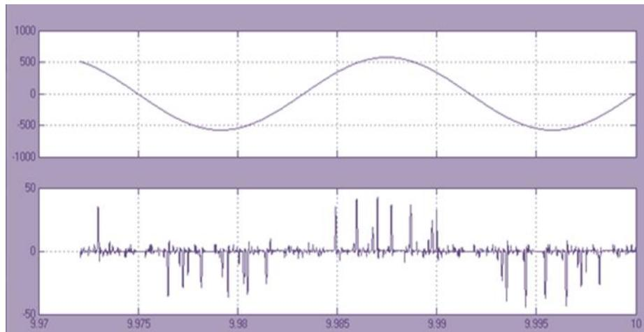
**Fig. 12:** The instantaneous voltage and current of phase 'a' under unbalanced voltage
