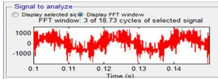
**Fig. 10:** Input current harmonics under balance voltage
