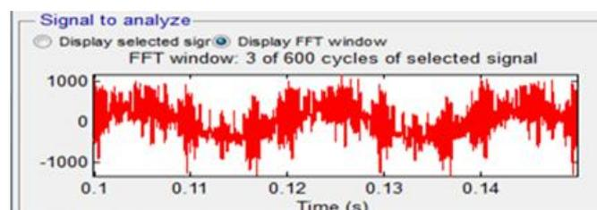
**Fig. 13:** The input current harmonics under utility voltage unbalance
