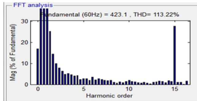
**Fig. 11:** FFT analysis of input current harmonics under balance voltage
