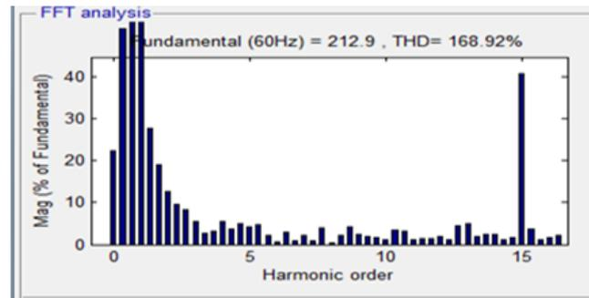
**Fig. 14:** FFT analysis of input current harmonics under utility voltage unbalance
