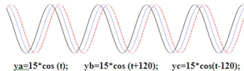
**Fig. 1:** The three phase balanced voltages
