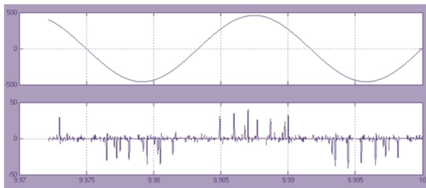
**Fig. 9:** The instantaneous voltage and current of phase 'a' under balanced voltage
