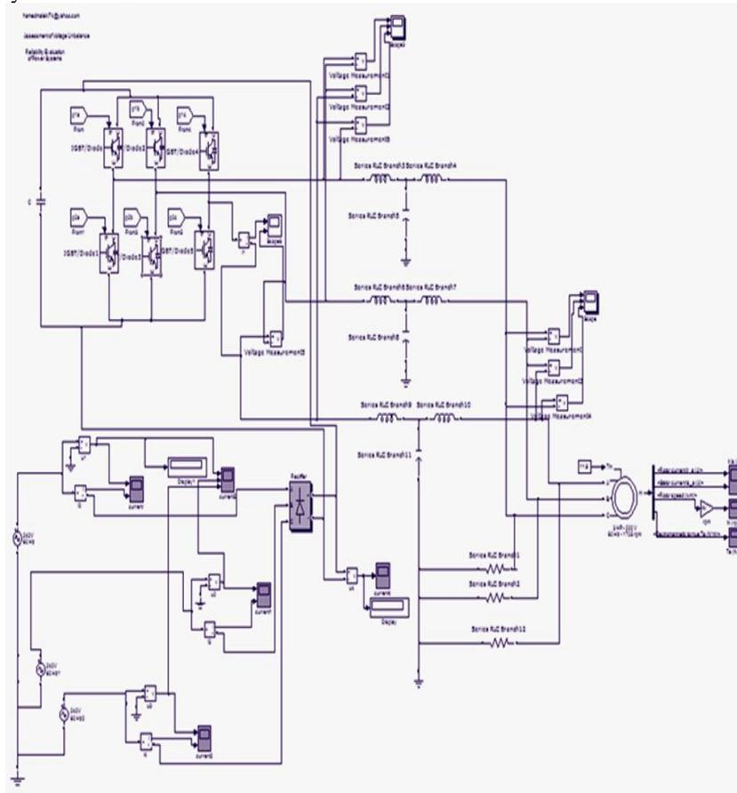
Fig. 7: The MATLAB/SIMULINK model of typical adjustable speed drive which feed with unbalanced voltages
