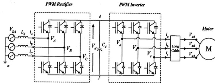
Fig. 6: ASD with PWM rectifier
