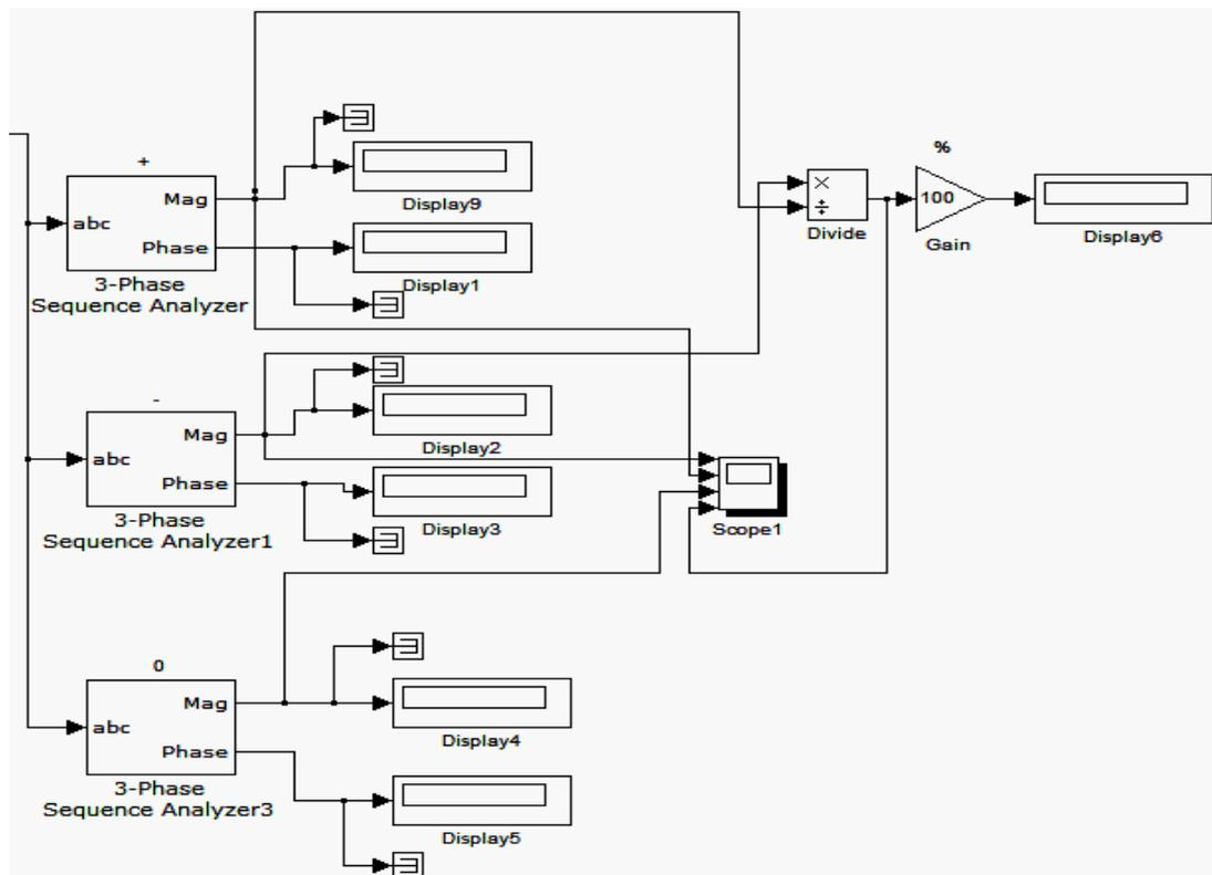
**Fig. 8:** Unbalance voltage degree measurement
