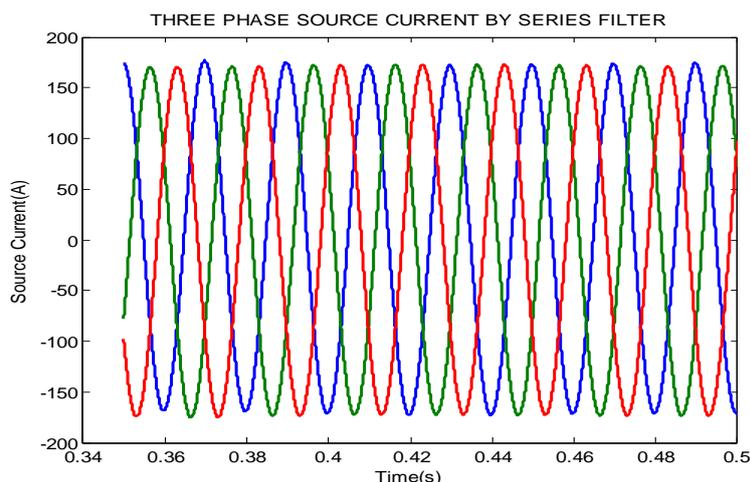
**Fig. 11:** Three phase source current with series active filters
