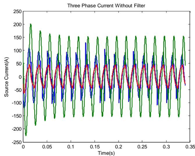
**Fig. 10:** The three phase source current without hybrid series active filter
