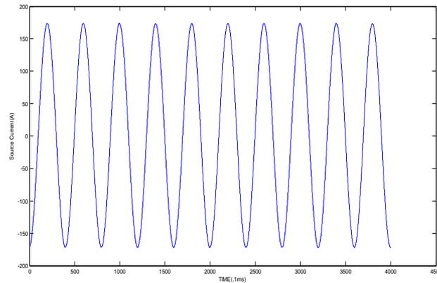
**Fig. 9:** The source current phase 'a' of balanced nonlinear load after compensation
