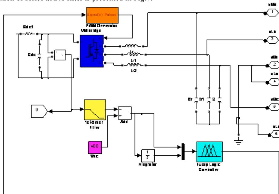
Fig. 7: The circuit of series active power filter
