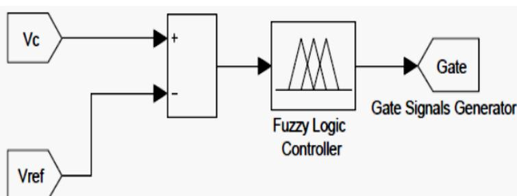
**Fig. 2:** Fuzzy controller structure block diagramThe main advantages of fuzzy control are its linguistic
