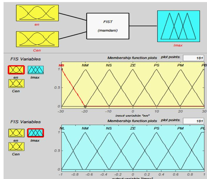
**Fig. 4:** the GUI interface of fuzzy logic controller setting in MATLAB
