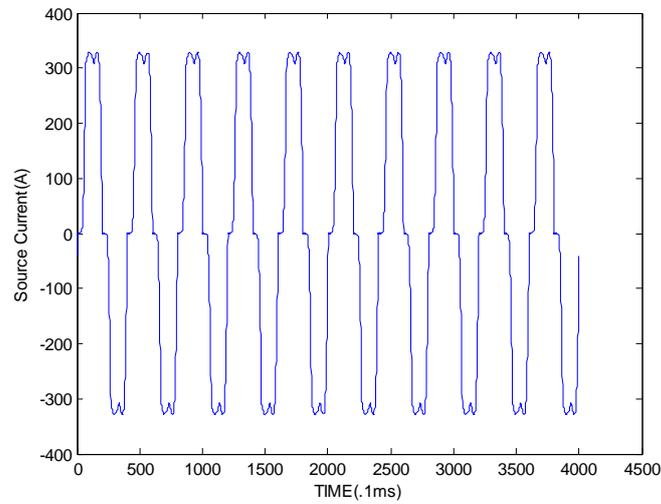
**Fig. 8:** The source current of phase 'a' of balanced nonlinear load without any compensation
