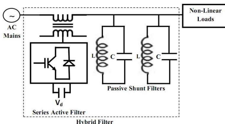
**Fig. 1:** basic configuration of hybrid filter
