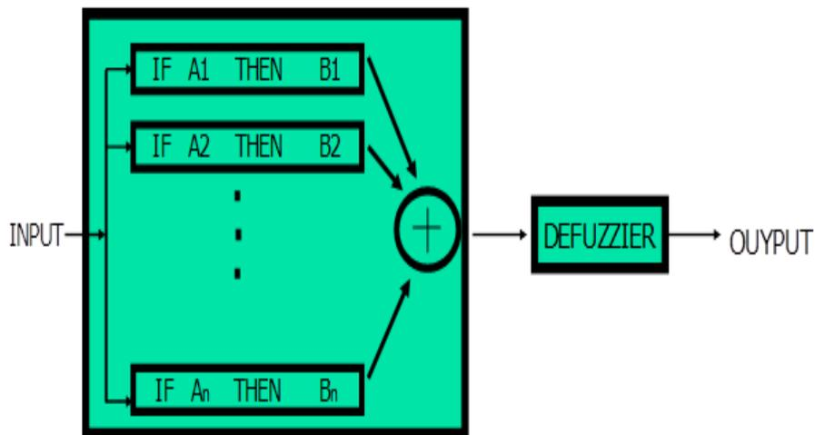
**Fig. 3:** the basic scheme of fuzzy logic controller
