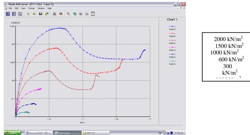
**Fig. 6:**  $q'$  vs. strain curve in sample SW in confinement pressure from 100 to 2000  $\text{kN/m}^2$ .
