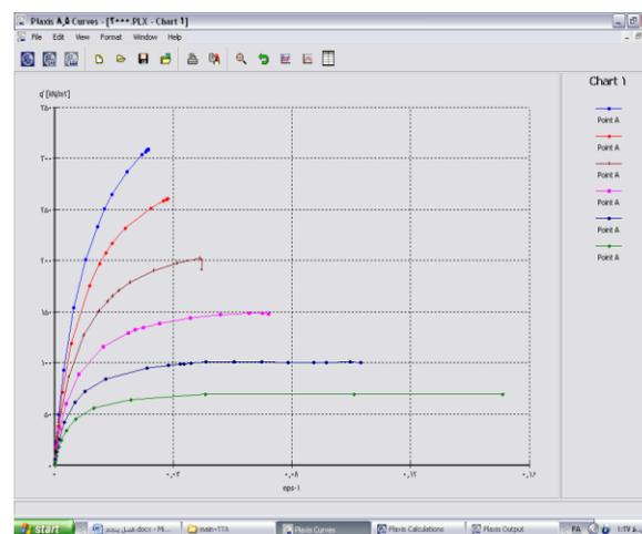
**Fig. 7:**  $Q'$  vs. strain curve in sample SC in confinement pressure from 100 to 2000  $\text{kN/m}^2$ .
