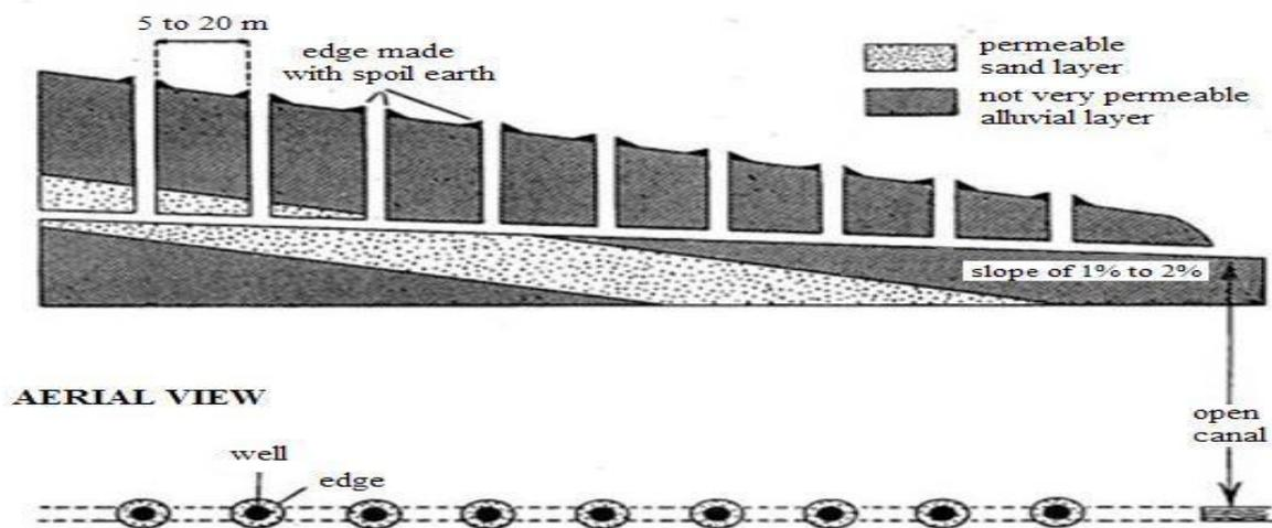
**Fig. 2:** Qanat's System Profile and Aerial View.
