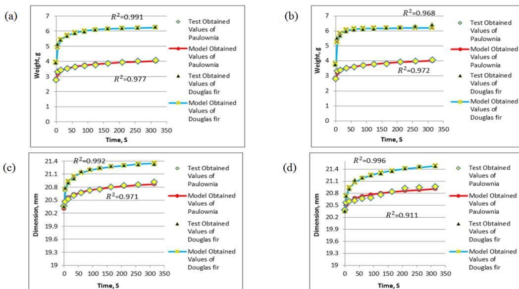
**Fig 3:** Weight changes in the radial (a) and tangential directions (b), and dimensions changes in the radial (c) and tangential directions (d) due to neutral liquor.
