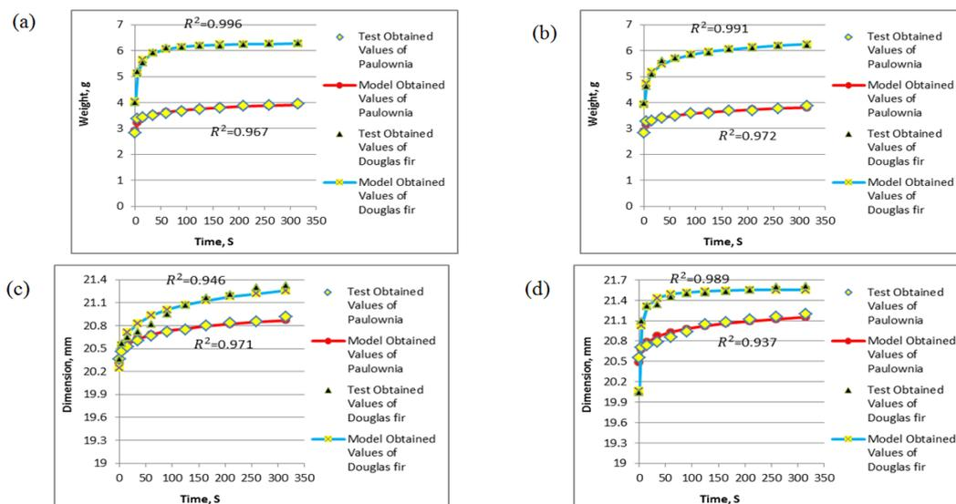
**Fig. 2:** Weight changes in the radial (a) and tangential directions (b), and dimensions changes in the radial (c) and tangential directions (d) due to alkaline liquor.
