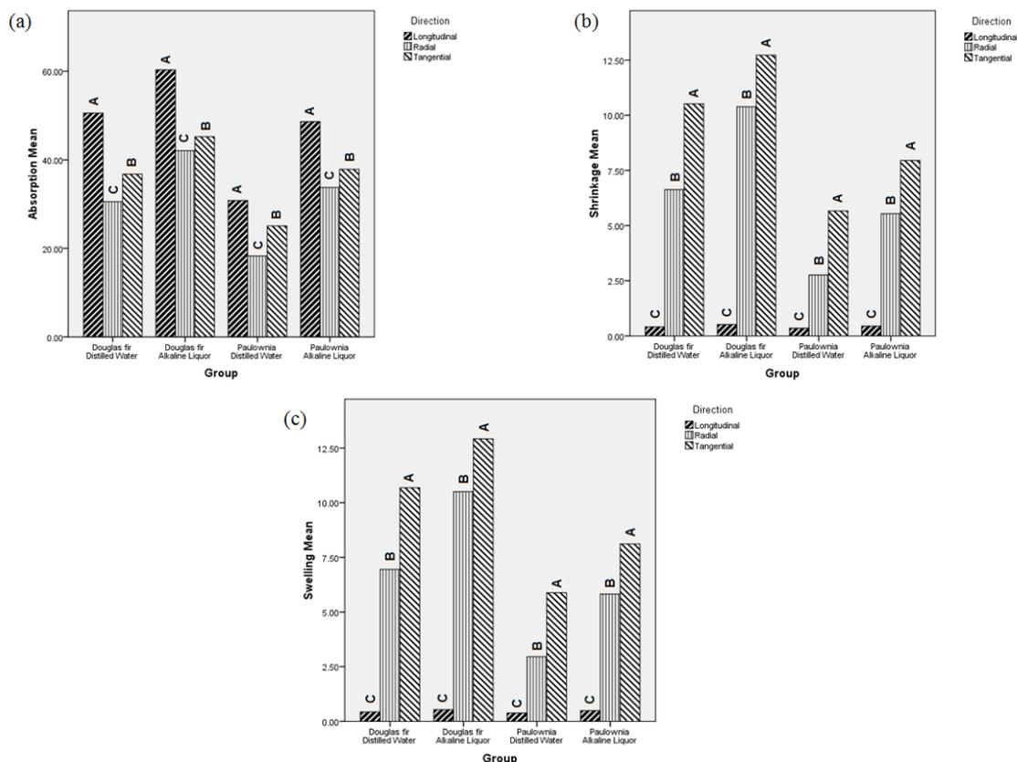
**Fig. 1:** The absorption (a), shrinkage (b) and swelling (c) in the longitudinal, radial and tangential directions due to neutral and alkaline liquors.
