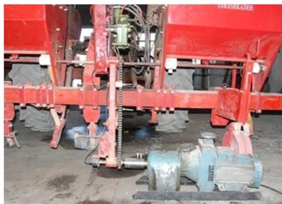
**Fig. 5:** Simulation of fertilizer applicator field operation conditions in workshop.
