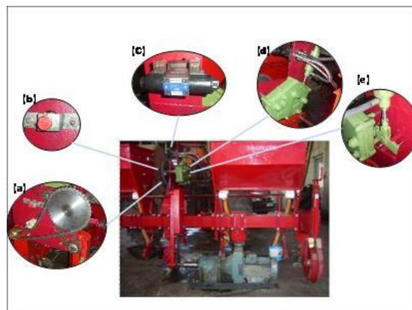
**Fig. 3:** Components for adjusting rotation speed of axles: (a) sprocket and chain unit (b) gear box lever position sensor (c) hydraulic flow control valve (d) gear box and hydraulic actuator of gear box lever (e) gear box lever.
