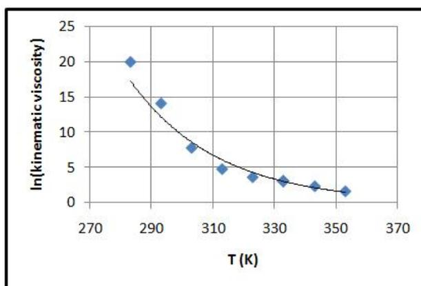
**Fig. 4:** Kinematic Viscosity of almond oil versus temperature.
