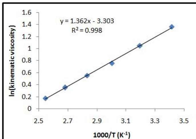
Fig. 7: Dependence of  $\log_e(\text{kinematic viscosity})$  versus  $1/T$  for diesel oil.
