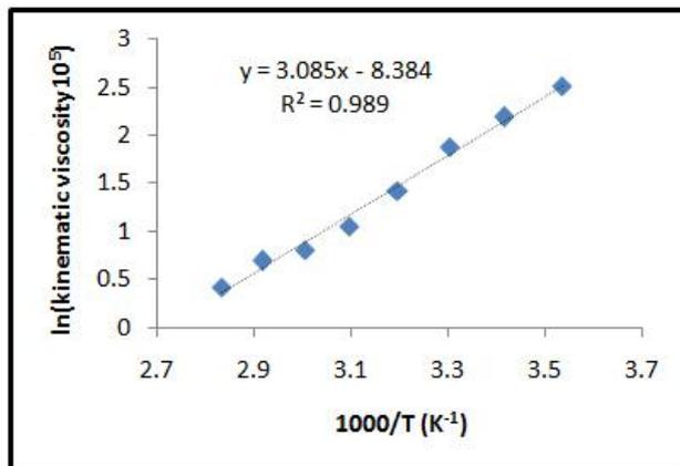
**Fig. 3:** Dependence of  $\log_e(\text{kinematic viscosity})$  versus  $1/T$  for Linseed vegetable oil.
