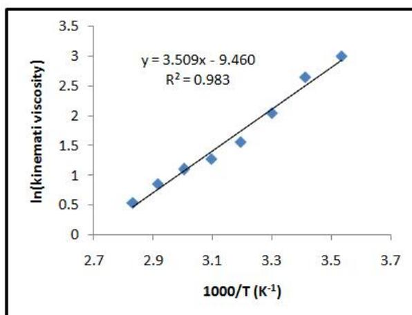
**Fig. 5:** Dependence of  $\log_e(\text{kinematic viscosity})$  versus  $1/T$  for almond vegetable oil.
