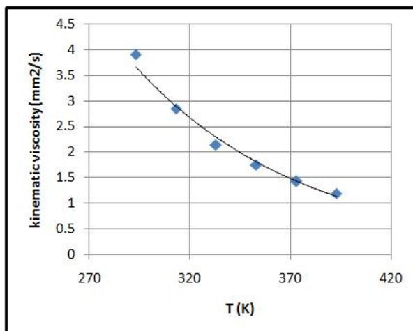
Fig. 6: Kinematic viscosity of diesel [13]
