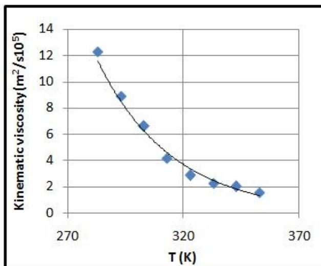
**Fig. 2:** Kinematic viscosity of linseed oil versus temperature.
