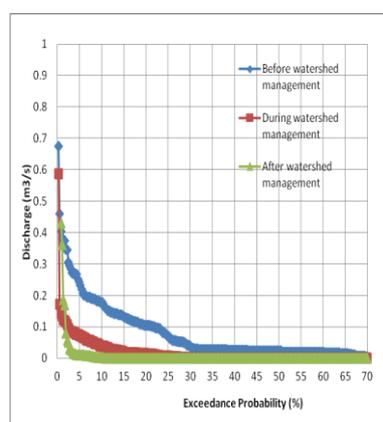
**Fig. 2:** Flow duration curve for the three study phases.
