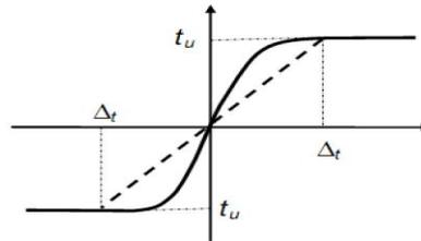
**Fig. 3:** Ideal behavioral curve of axial soil spring.
