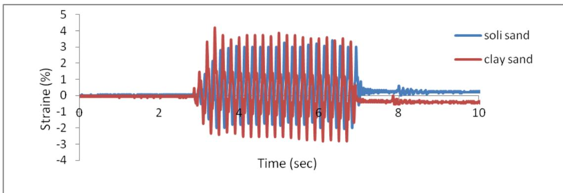
**Fig. 15:** Comparisons of pipe strains under cyclic charge in two types of construction and clay sand soils
