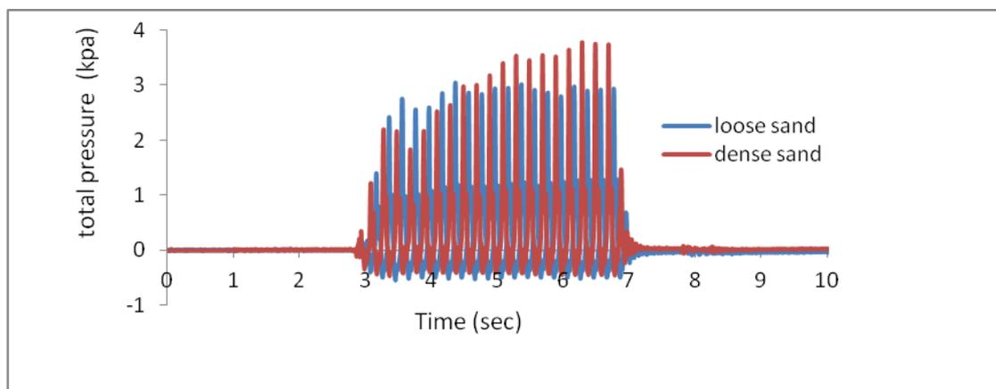
**Fig. 11:** Comparison of incurred force on pipe for loose and dense sand.
