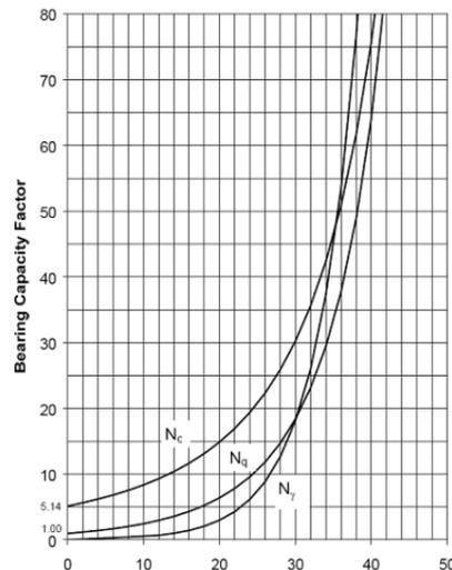
**Fig. 6:** Cohesive soil resistance ratios for various values of soil friction.
