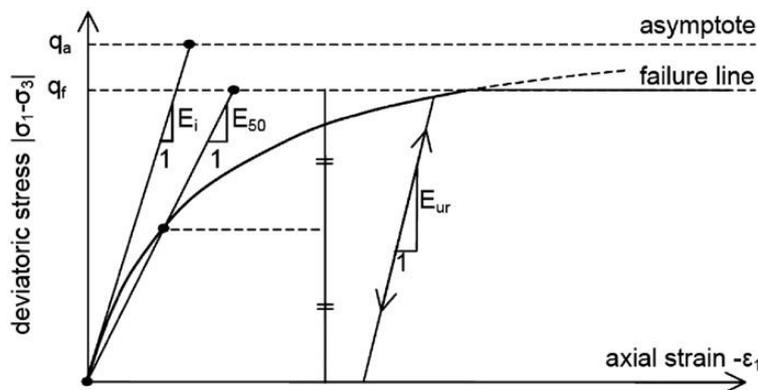
Fig. 9: Hardening soil model parameters.
