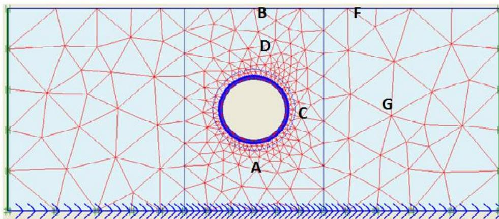
**Fig. 7:** Finite element model of buried pipe with 15 nodal element meshing.
