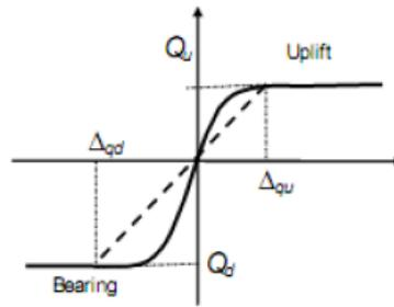
**Fig. 5:** Ideal curve for soil vertical springs.
