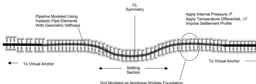
**Fig. 2:** Modeled soil with Winkler non-linear springs [1].
