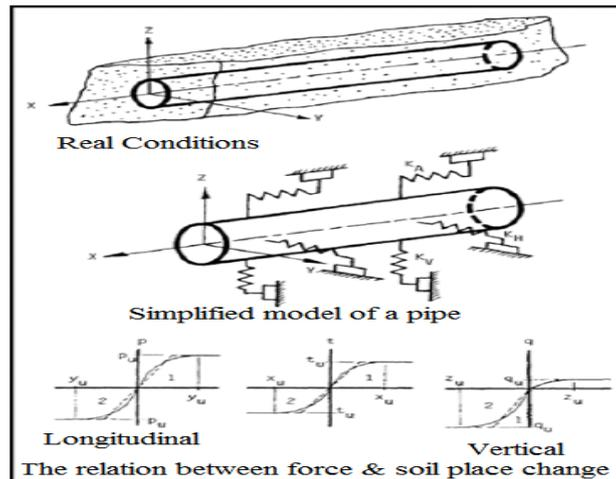
**Fig. 1:** Finite element (beam type) of buried pipe with soil and supports.
