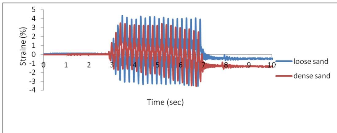
**Fig. 10:** Comparing strains on pipe in loose and dense sand.
