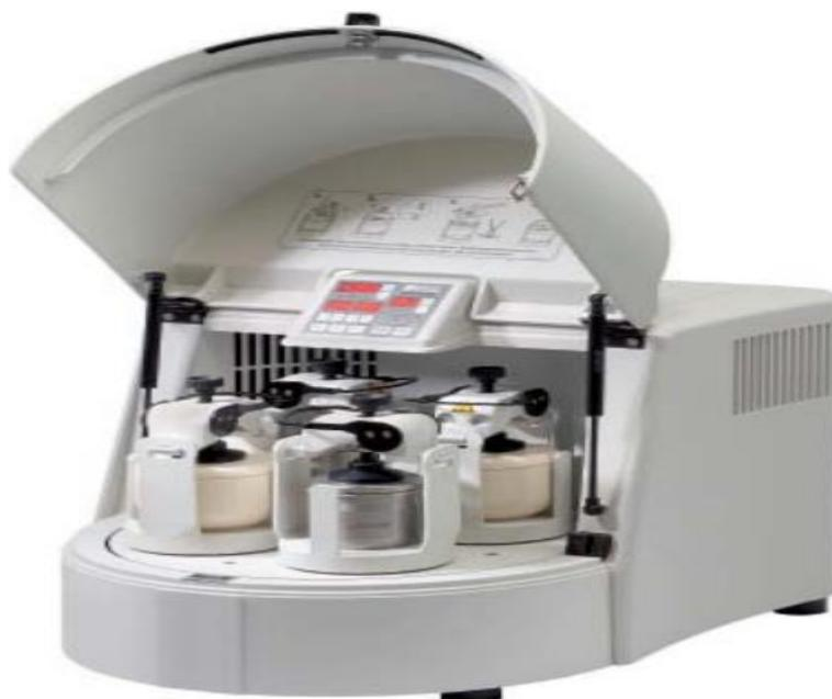
FRITSCH Planetary Mill PULVERISETTE 5 classic line (Image courtesy of FRITSCH GMBH) [29]
