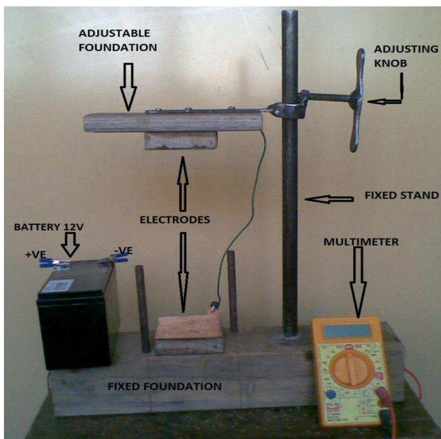
**Fig. 3:** Experimental Setup for Measuring Current Measurement
