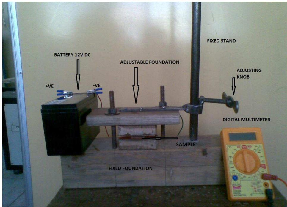
Fig. 4: Experimental set-up of electrical current measurement (with sample)
