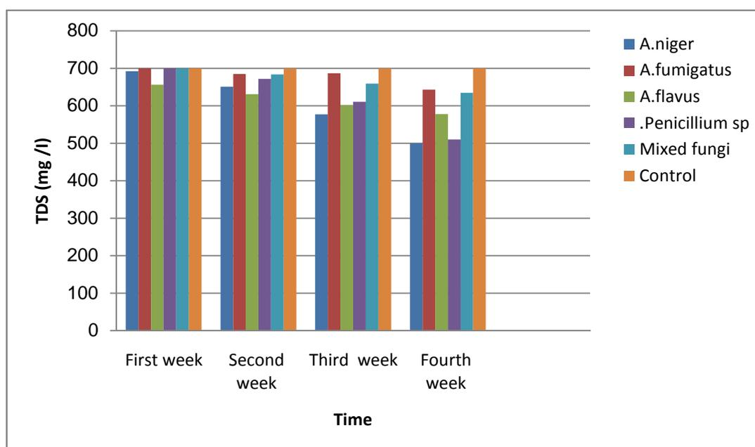
**Fig. 1:** Values of Total Dissolved Solid ( TDS ) in wastewater treatment with 10 c<sup>o</sup>, pH 2 and 0.0 gm / l NaCl.
