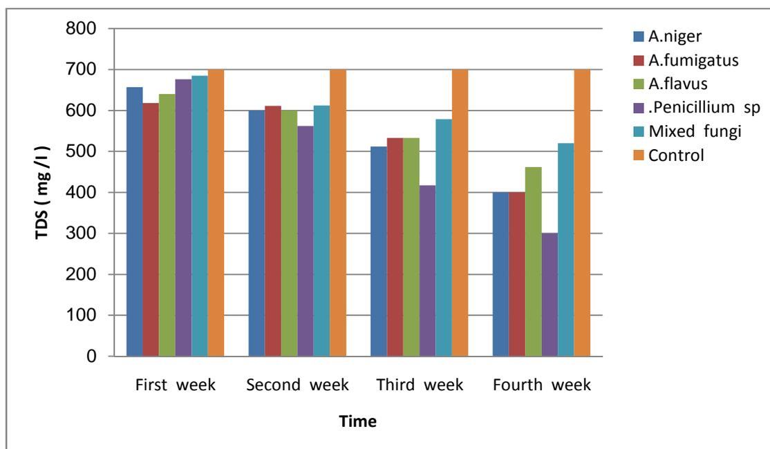
**Fig. 3:** Values of Total Dissolved Solid ( TDS ) in wastewater treatment with 30 c<sup>o</sup>, pH 6 and 1.0 gm / l NaCl.
