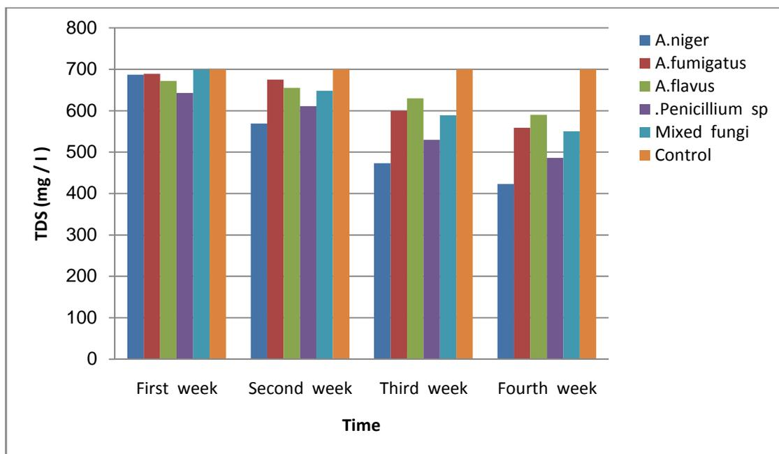
**Fig. 4:** Values of Total Dissolved Solid ( TDS ) in wastewater treatment with 40 c<sup>o</sup>, pH 8 and 2 gm / l NaCl.
