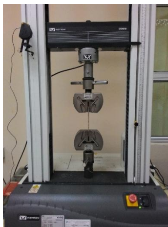
Fig. 2: Universal INSTRON model 3369 machine.
