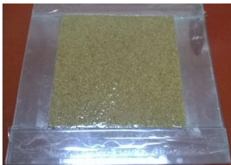
Fig. 1: Natural fiber reinforced epoxy in a glass mould.
