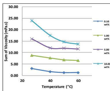
**Fig. 3:** Viscosity of nanofluids at different temperature.
