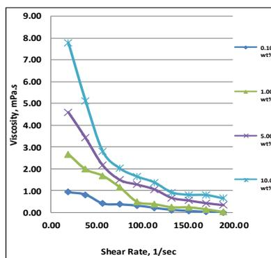
**Fig. 2:** Viscosity of nanofluids at 27°C.
