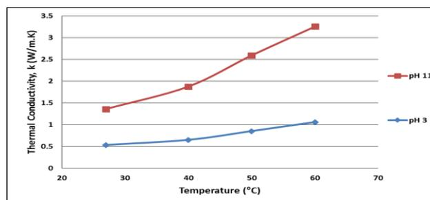
**Figure 5.** Thermal conductivity of TiO<sub>2</sub>-DW base fluid at different pH.
