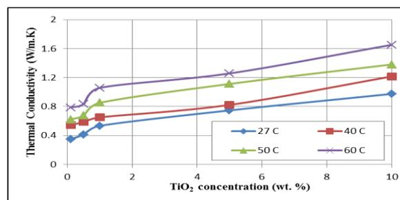
**Fig. 4:** Thermal conductivity of nanofluids at different temperatures.
