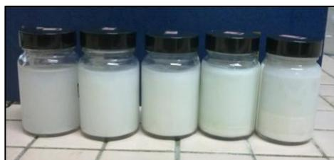
**Fig. 1:** Samples of  $\text{TiO}_2$ -DW based nanofluids with PVP.
