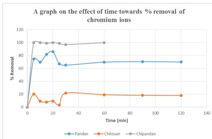
**Fig. 2:** The effect of contact time towards % removal of chromium ions
