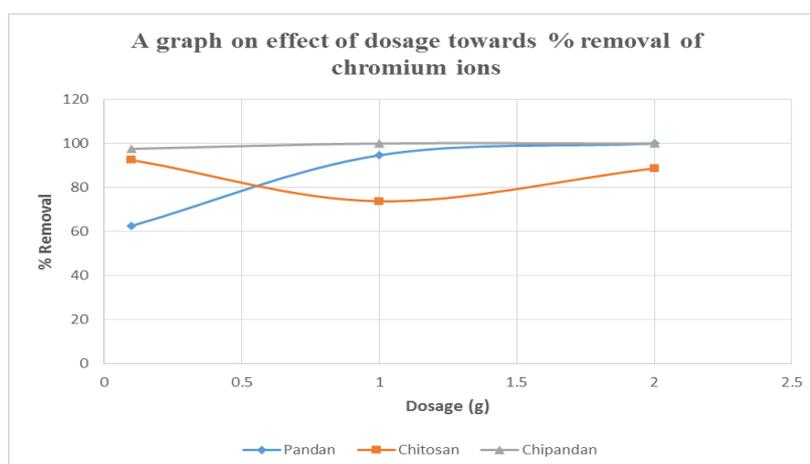
**Fig. 5:** The effect of dosage biosorbent towards % removal of chromium ions
