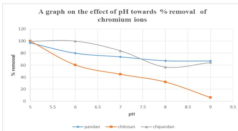
**Fig. 4:** The effect of pH solution towards % removal of chromium ions
