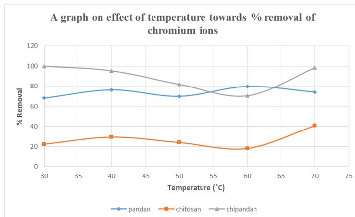
**Fig. 3:** The effect of temperature towards % removal of chromium ions
