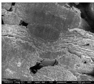
**Fig. 2:** Micrographs of a cross section at density  $500 \text{ kg m}^{-3}$  OPEFB composite boards with resin content 10% at 500x magnification.
