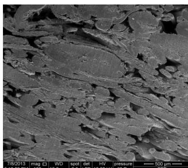
**Fig. 1:** Micrographs of a cross section at density  $500 \text{ kg m}^{-3}$  OPEFB composite boards with resin content 10% at 100x magnification.
