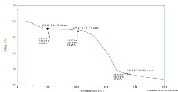
**Fig. 3:** TGA properties of OPEFB composite boards.
