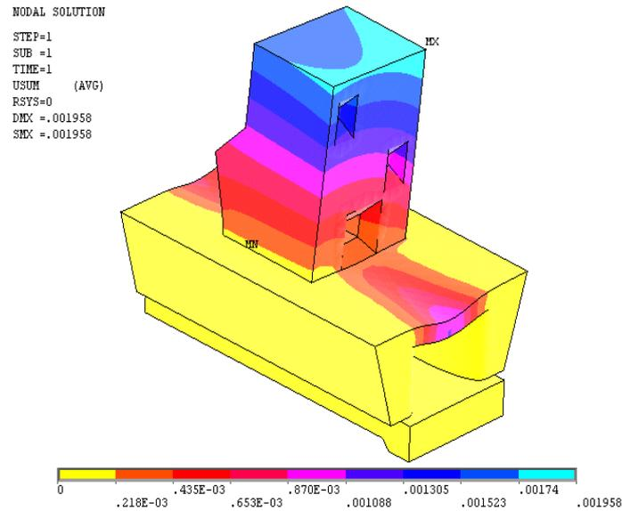
**Fig. 4:** Distribution of intake tower displacement-static.
