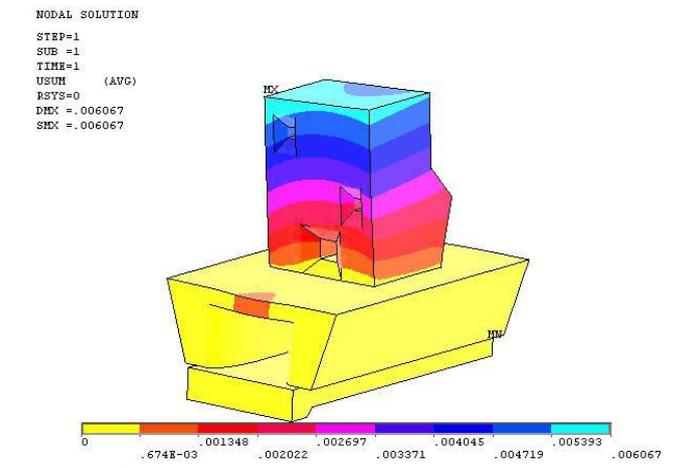
**Fig. 5:** Distribution of intake tower displacement- dynamic X.
