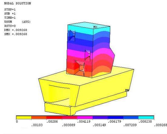
**Fig. 6:** Distribution of intake tower displacement- dynamic Y.
