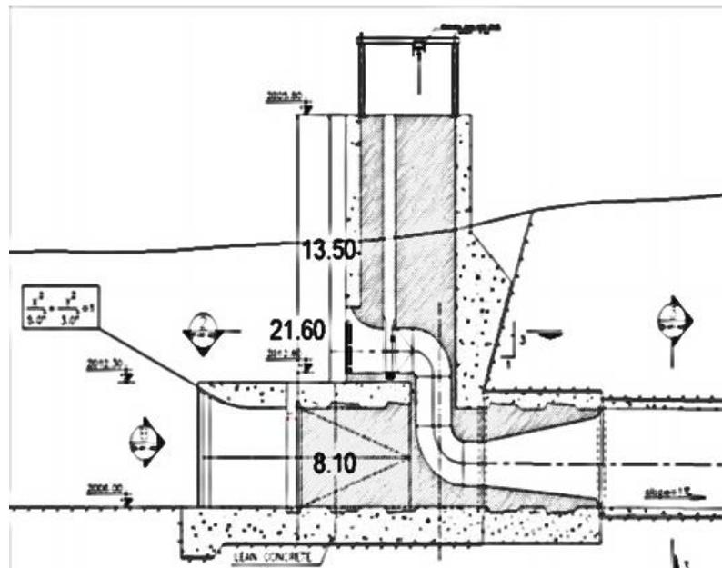
**Fig. 1:** Geometric dimensions of the studied intake tower.
