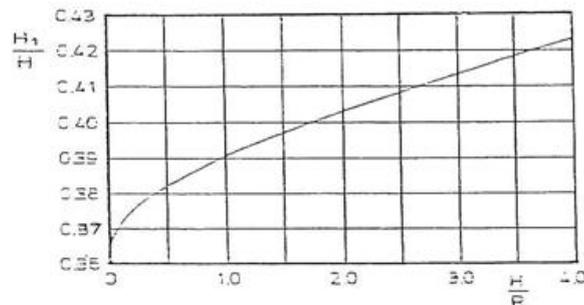
**Fig. 3:** The effect point of hydrodynamic force.
