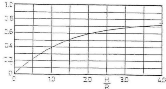
**Fig. 2:** Correction coefficient of hydrodynamic force.
