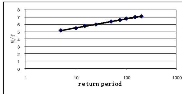
**Fig. 2:** The curve of earthquake return period and magnitude  $M_s$  in an area with the radius of 250 km from Behbahan using Gutenberg-Richter function.
