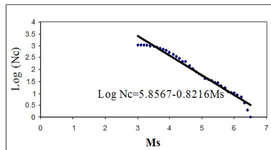
**Fig. 1:** The linear relationship between frequency and magnitude of the earthquakes in the range of 250 km from Behbahan.
