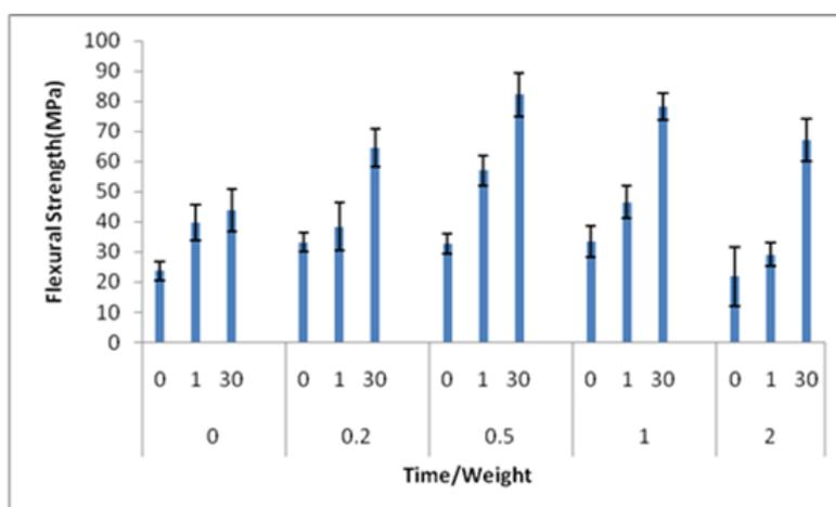
**Fig. 1:** Mean and standard deviation of flexural strength for different weight groups in three testing times.
