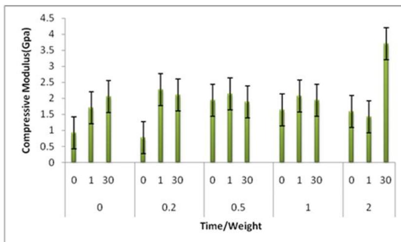
**Fig. 4:** Mean and standard deviation of compressive modulus for different weight groups in three testing times.
