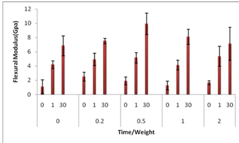
**Fig. 2:** Mean and standard deviation of flexural modulus for different weight groups in three testing times.
