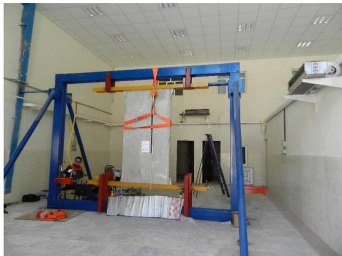
**Fig. 2:** Locating the wall on the laboratory frame.
