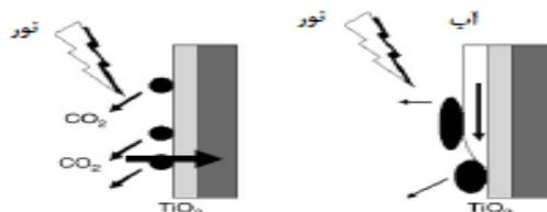
**Fig. 1:** schematic representation of self-cleaning mechanism from the hydrophilic surface of titanium dioxide.
