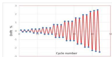
**Fig. 5:** cyclic loading in terms of the criteria of AISC2005 regulations (8).
