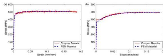
**Fig. 4:** The stress-strain curve of the steel in the model test by Berman and Bärnau, a) link beam flange and the other members and b) the center of linking bar [7].
