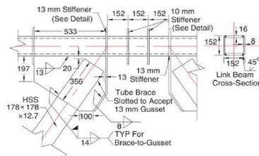
**Fig. 2:** Details of the test model by Berman and Bärnau [7].
