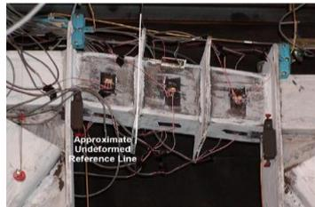
**Fig. 3:** the rupture of connection link and in the experiment model by Berman and Bärnau [7].
