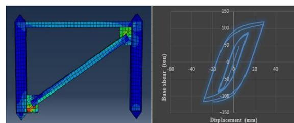
**Fig. 8:** The results of the frame analysis with single-diagonal bracing, a) displacement hysteresis curve above the frame in front of the base shear) deformation model for the frame.
