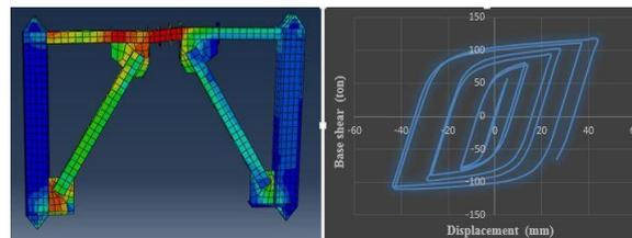
**Fig. 7:** results of frame analysis with divergent bracing, A) displacement hysteresis curve of the frame in front of the base shear) deformation model of the frame
