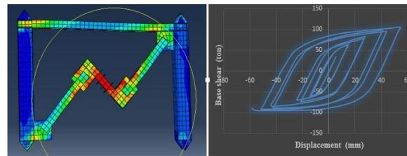
**Fig. 9:** results of frame analysis with the proposed bracing, a) displacement hysteresis curve of the frame in front of the base shear, B) deformation model of the frame.
