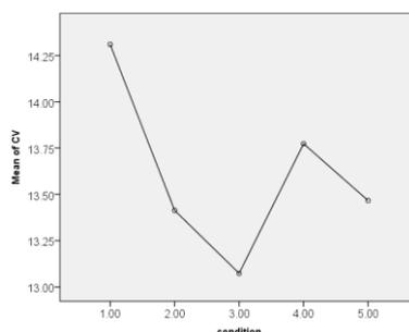
**Fig. 8:** Changes in non-uniformity index for viscose polyester yarns samples at a ratio of 80/20.
