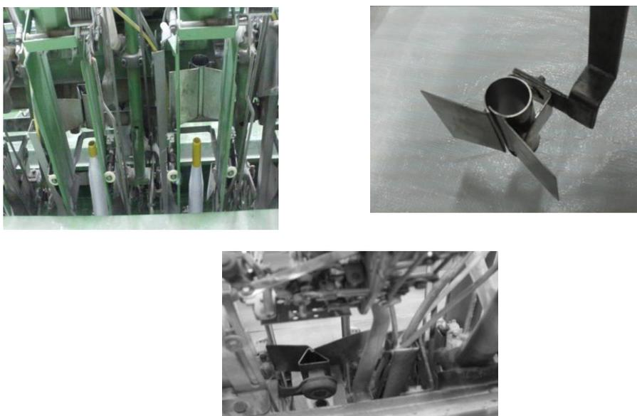
**Fig. 5:** Balcony made a - b and the original one made by SCHLAFHORST Company.
