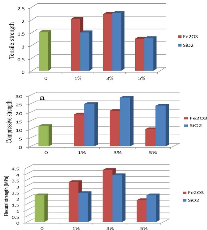
**Fig. 1:** (a) Compressive strength, (b) Tensile strength, and (c) Flexural strength of samples
