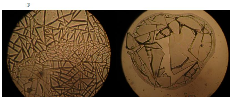
Fig. 4: sample dried by hot plate (right side) – sample dried in the air (left side).
