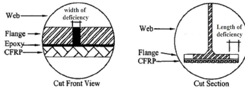
**Fig. 2:** Schematic of deficiencies in bottom flange.
