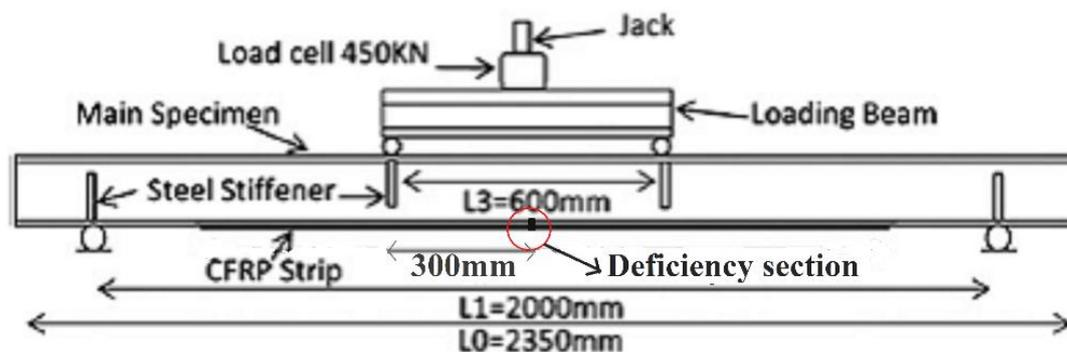
Fig. 1: Steel beams dimensions and location of deficiency.
