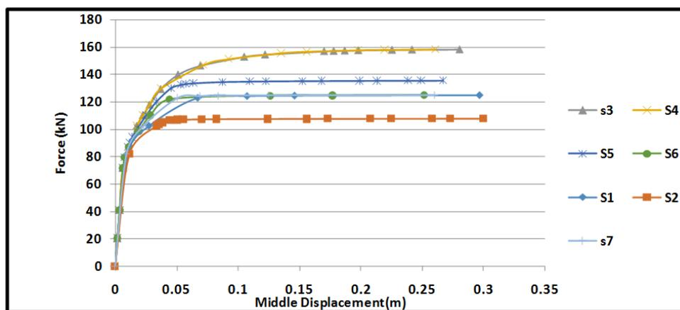
Fig. 6: Force- Displacement diagram for the middle of flange.
