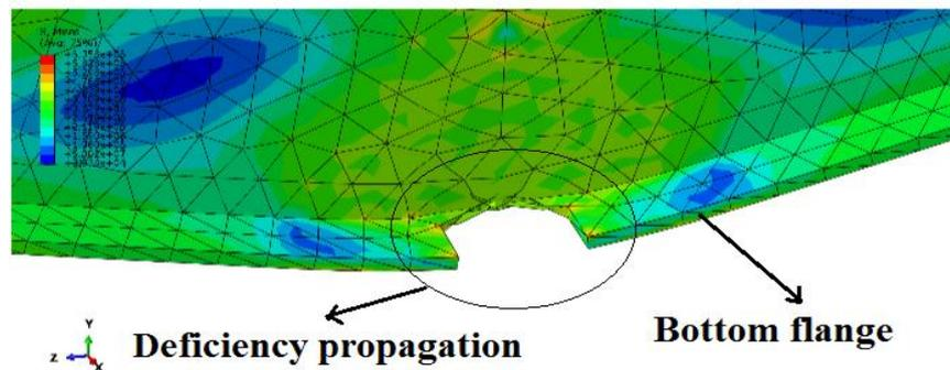
Fig. 5: Deficiency Propagation in tensile flange of non-strengthened beam.
