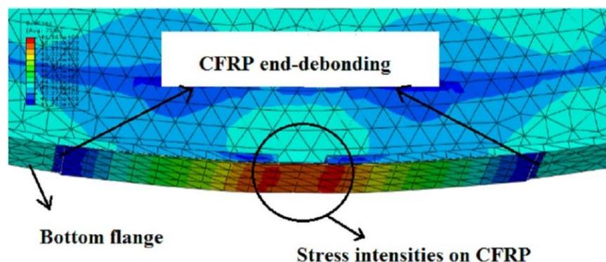
Fig. 7: End-debonding of CFRP at the tip of plate and stress intensity on CFRP at the deficiency area.
