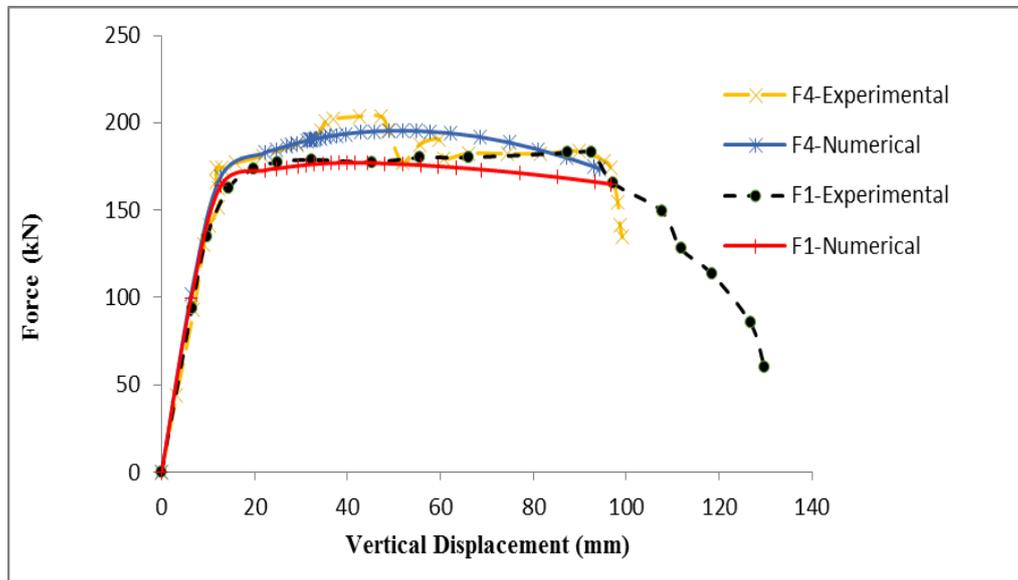
**Fig. 3:** Validation of vertical displacement at the mid-span (experimental and numerical).
