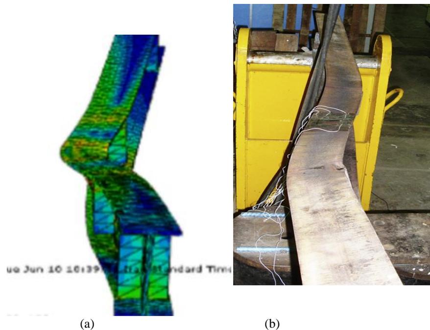
**Fig. 4:** Lateral-torsion-buckling (a) numerical (this research), (b) tested beam [15].
