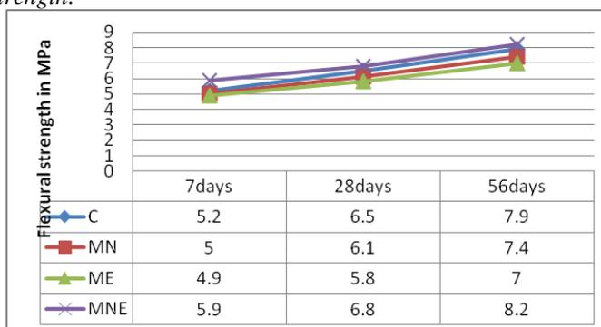
**Fig. 2:** Shows the Flexural Strength of samples at different ages in MPa.
