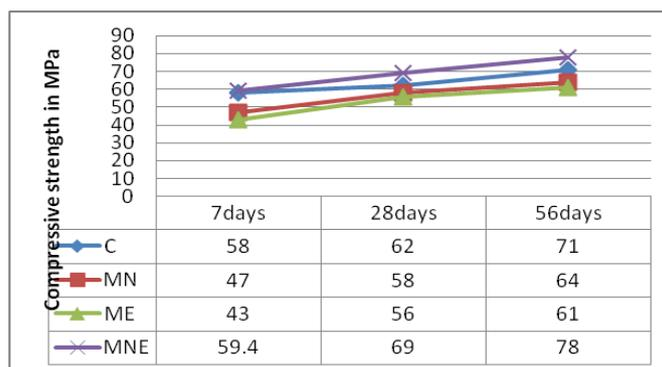
**Fig. 1:** Shows the Compressive strength of samples at different ages in MPa.
