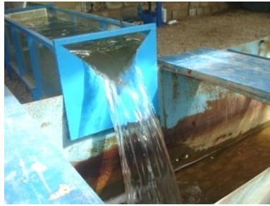
**Fig. 2.90:** degrees spillway of measuring output discharge from vortex tube.
