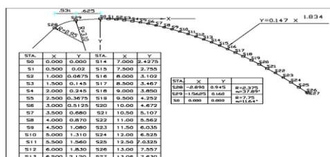
**Fig. 2:** Details of the Ridge and Spillway Form (Mollasadra Dam report).
