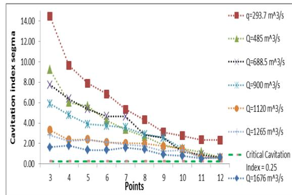
**Fig. 9:** Variations of Corrosion (Cavitation) Coefficient on the Spillway.
