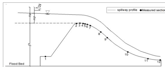
**Fig. 5:** Piezometer Locations on the Spillway (to 1:40 Scale).
