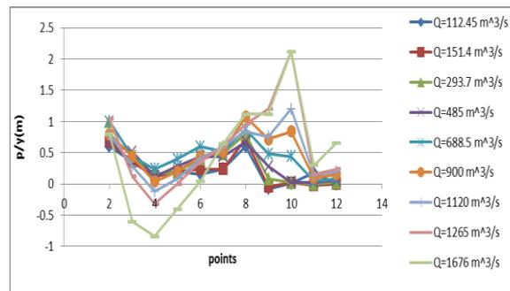
**Fig. 7:** Static Pressure Variations over the Mollasadra Dam Spillway Model.
