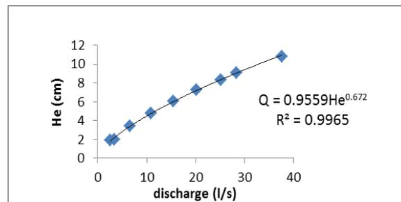
**Fig. 6:** Flow rate - Ogee Weir Scale Diagram.
