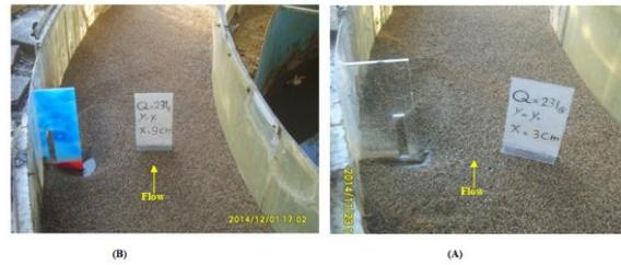
**Fig. 3:** Scour pattern at the end of a test. (A) Model A1 (B) Model A4.
